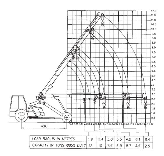
Rated loads are calculated for operation on leveled surface.
